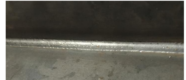
Fillet Welds "No Stop/Starts"
